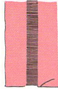
Correct Needle Thread Tension
