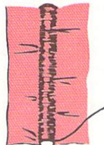
Tight Needle Thread Tension
