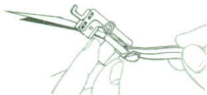
FIG. 72. INSERTING FOLDED BINDING IN OUTSIDE SLOT.
