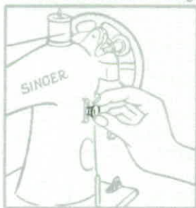
FIG. 43. STITCH REGULATING SCREW ON SINGER 15K26 AND 15K80 MACHINES.
